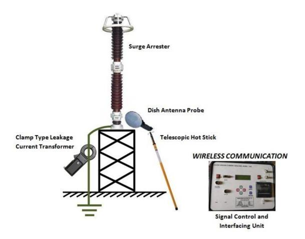
Beacon make **Wireless Leakage Current Analyzer** is a state of the art Portable On-line test system for Condition Monitoring, Residual Life Assessment and Health Check of Metal Oxide Surge / Lightning Arrestors without any interruption of service operation. The system provides immediate assessment of condition of Surge Arrestors through direct display of the 3rd harmonic resistive leakage current and total leakage current in micro-ampere.
